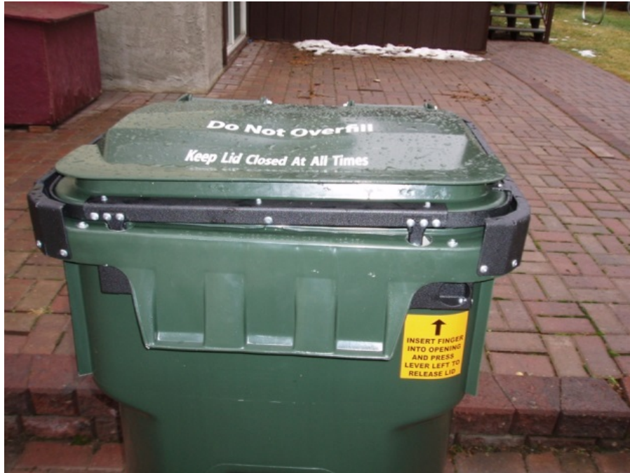
Figure 6. BearSaver bin with right side latch not securing lid.
