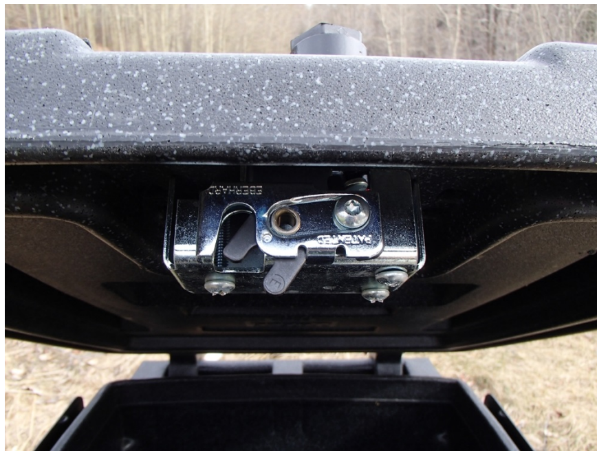
Figure 8. Latch mechanism inside lid of Bearicuda Stealth II bin.
